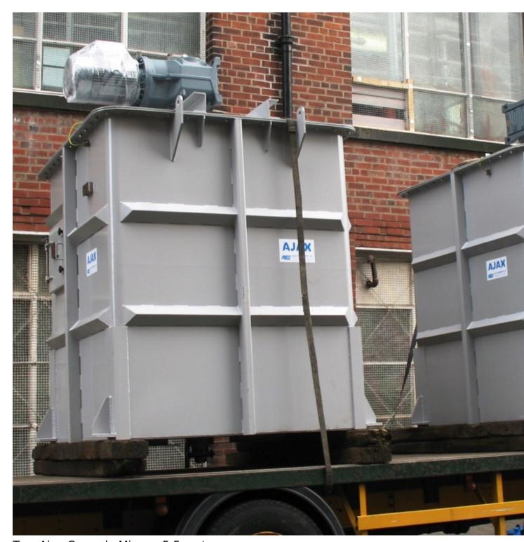
Two Ajax Cascade Mixers, 5.5 metre cube capacity site rated Atex zone 21, internal Zone 22.
