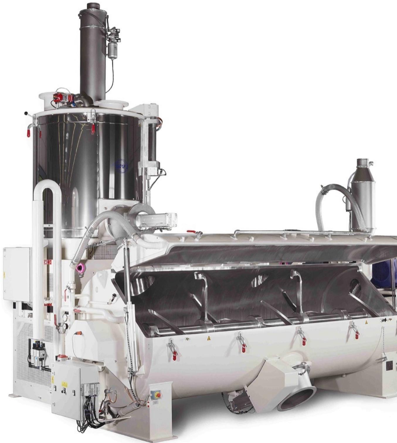
At NPE 2018, MTI Mischtechnik exhibits a Heating/Cooling Mixer Combination MTI Flex®-line that impresses with its outstanding dimensions. The type M 2000 / K 8000 unit features an 8,000 liter cooling vessel while measuring over 7 m (23 ft) in length and close to
