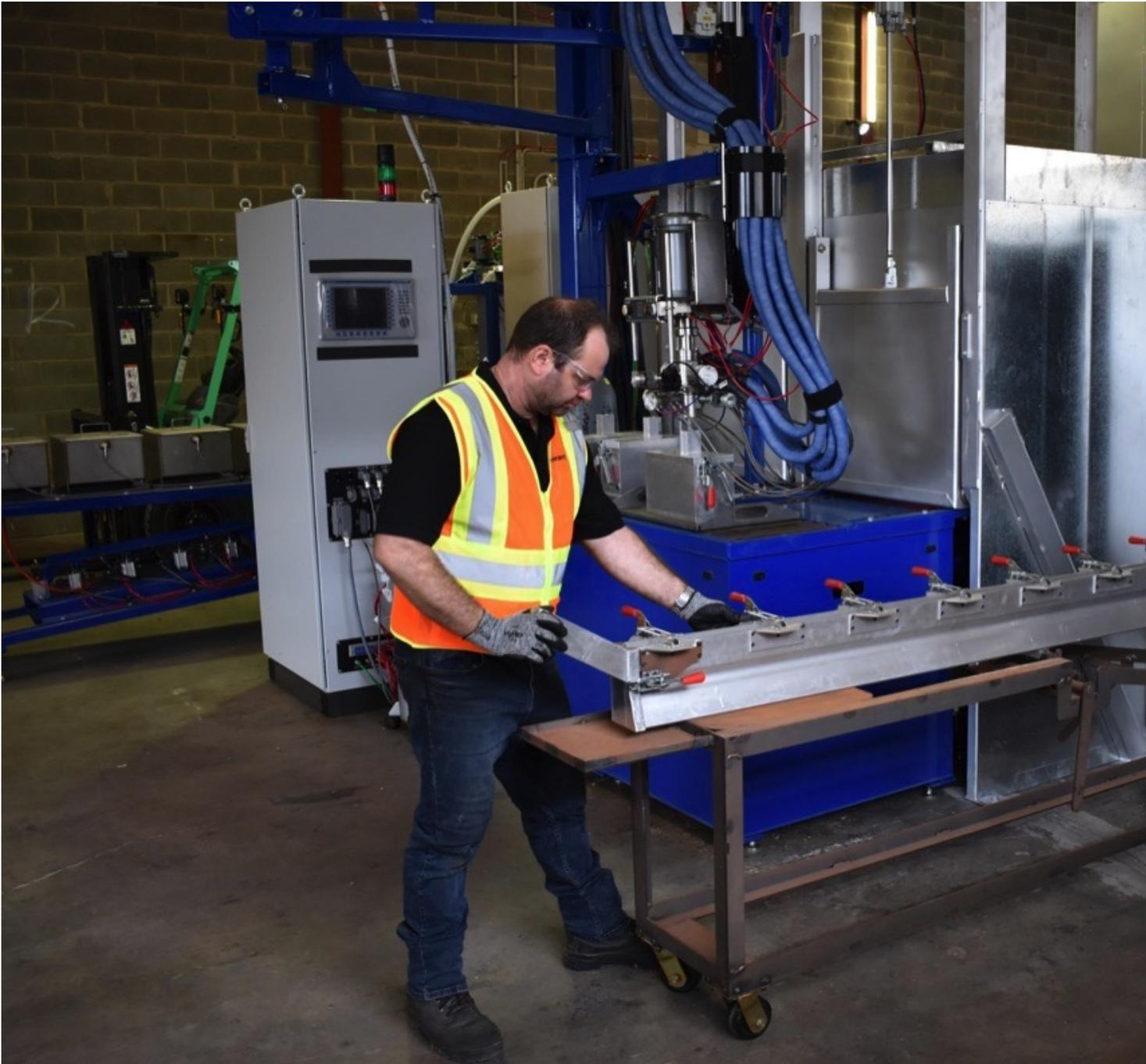
A urethane-filled mold is loaded into the curing oven.
