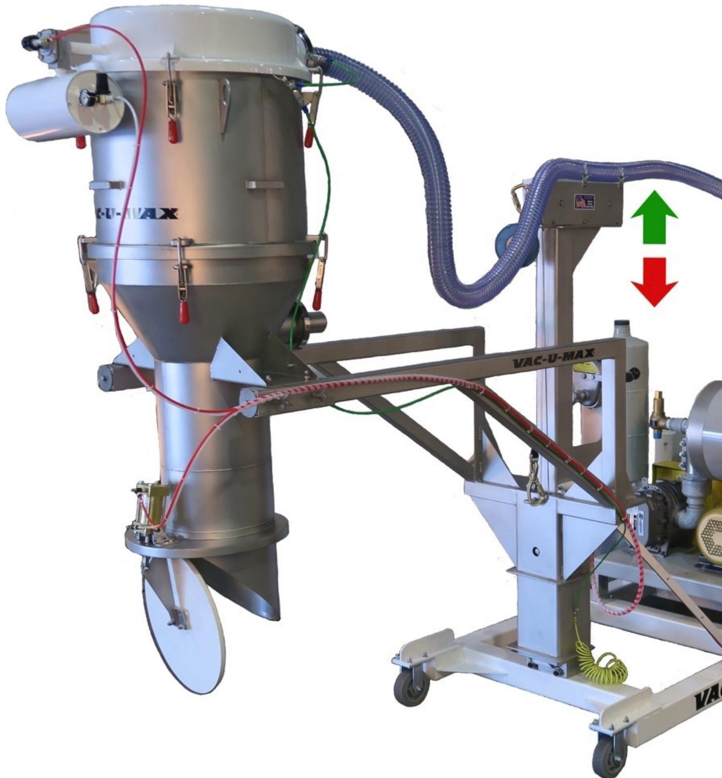
VAC-U-MAX Mobile Vacuum Conveying Systems offer ease-of-mobility for applications requiring access to tanks or other hard-to-reach processing areas. (Picture: VAC-U-MAX)
