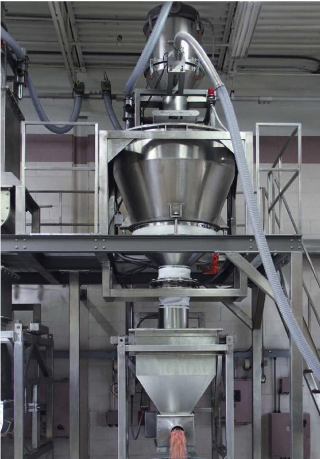
The VAC-U-MAX receiver always maintains a charge of material ready for dispensing. (Picture: VAC-U-MAX)
