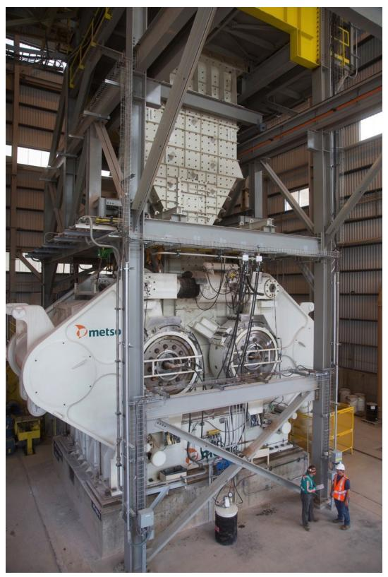
A featured solution at Expomin 2018, Metso's HRC3000 high-pressure grinding roll is more energy-efficient than traditional HPGRs. In the second half of 2017, the solutions reached a milestone of one hundred million short tons of crushed ore at Freeport-
