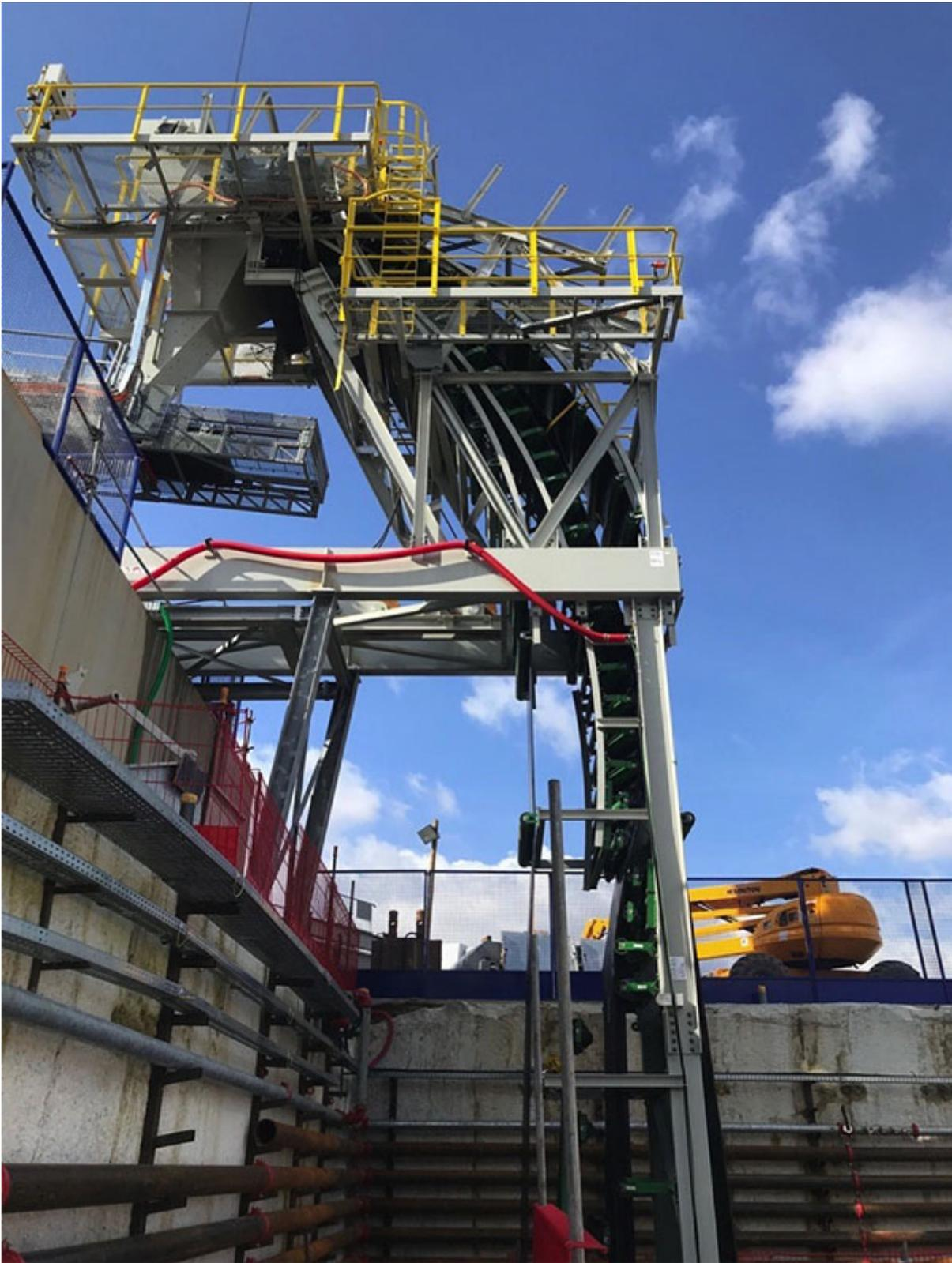
The DSI Sandwich belt high angle conveyor will elevate 800 t/h of tunnel muck at a 90° angle.
