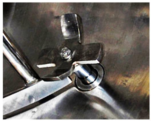
The paddle agitator forces material into the path of the tulip-style, high speed choppers, breaking down agglomerates and lumps for dispersion into the batch.
