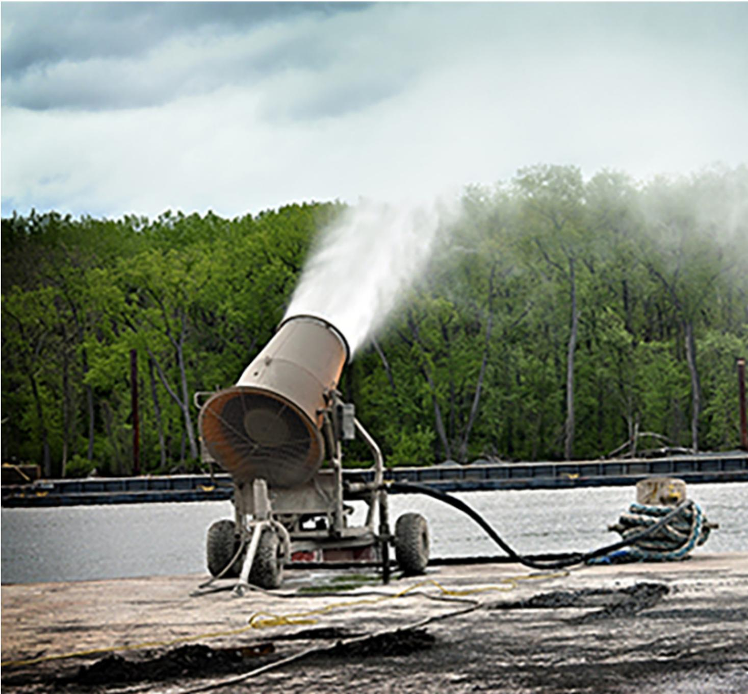
The unit features a 200-foot reach, 359° oscillation and 50° vertical adjustment angle.
