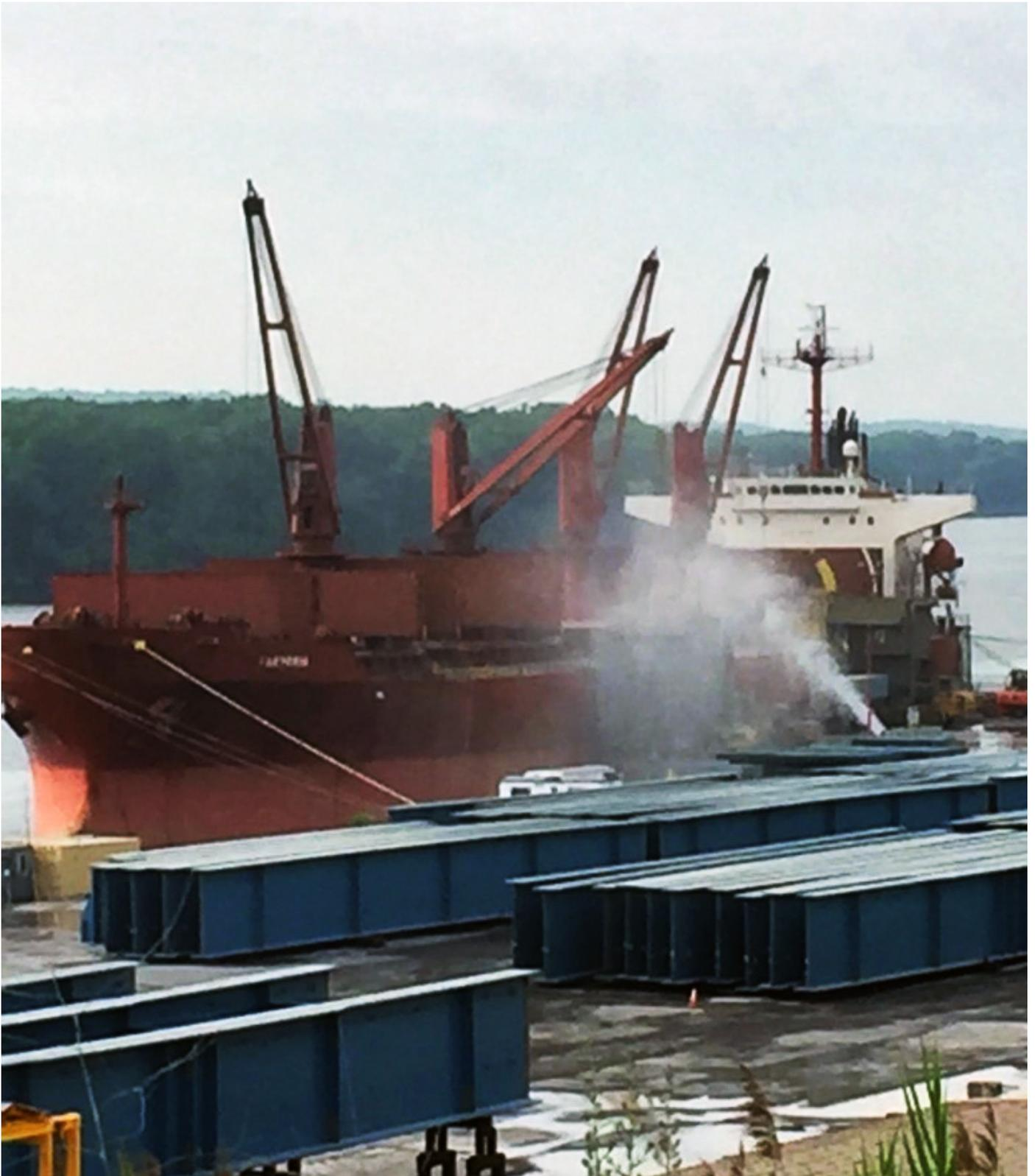
Dust suppression is directed where it is needed most in the unloading process.
