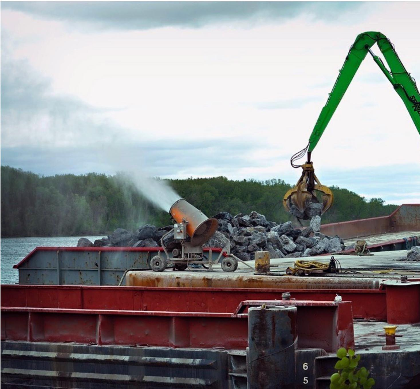
The mist can be seen stretching across the deck to deliver efficient dust suppression.
