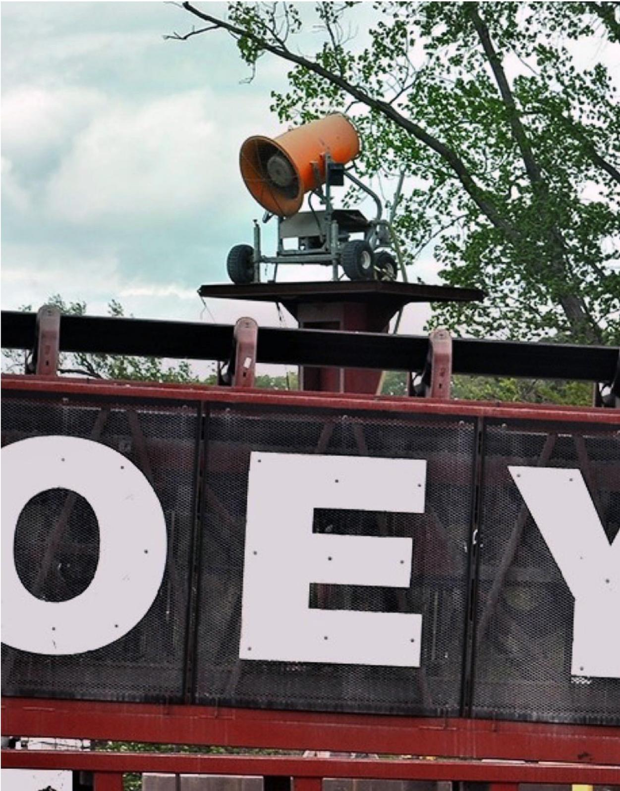
Mounted on a tower, the DB-60 suppresses dust over metal scrap recycling piles.
