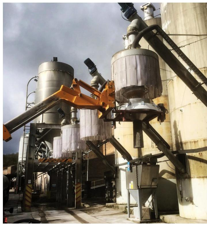
The sieve unit is transported and elevated into position above the tanker using a telescopic handler.
