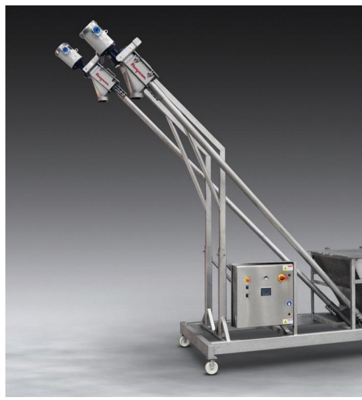
Twin BEV-CON Flexible Screw Conveyor system with common hopper and mobile base transfers difficult-to-convey materials and blends at multiple plant locations, and can be rolled to a wash-down station for sanitising.
