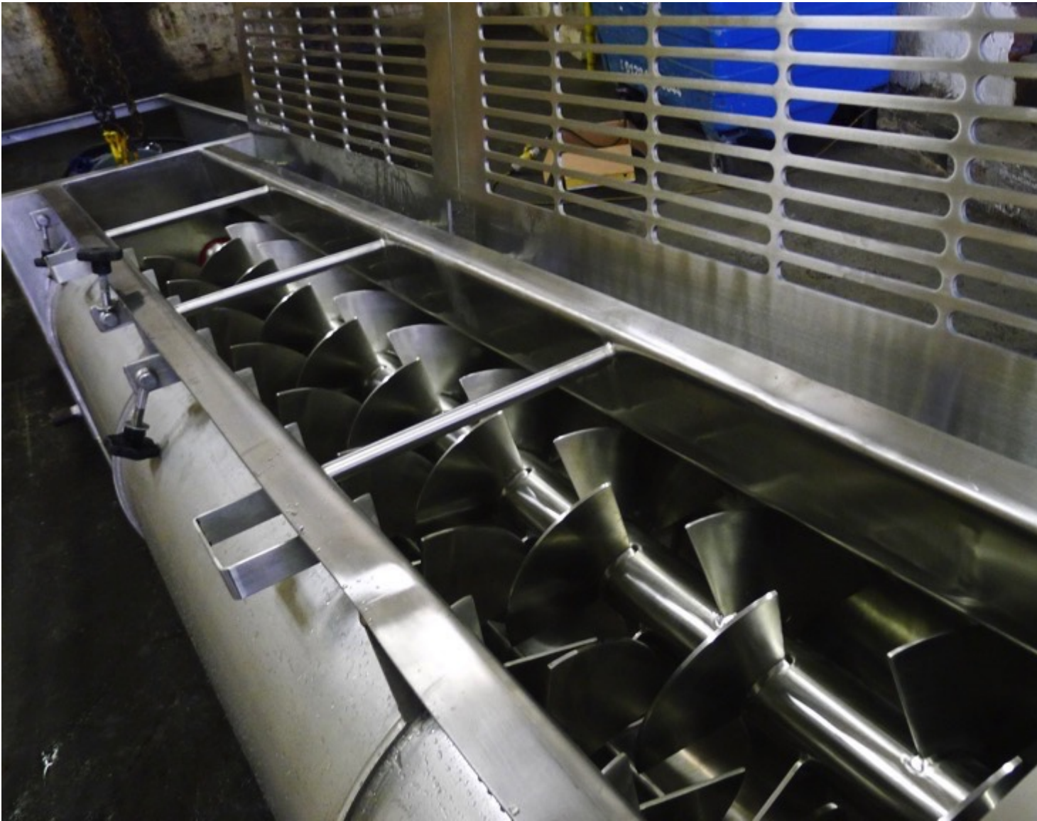
Ajax mixers for production of potato products at Agristo.
