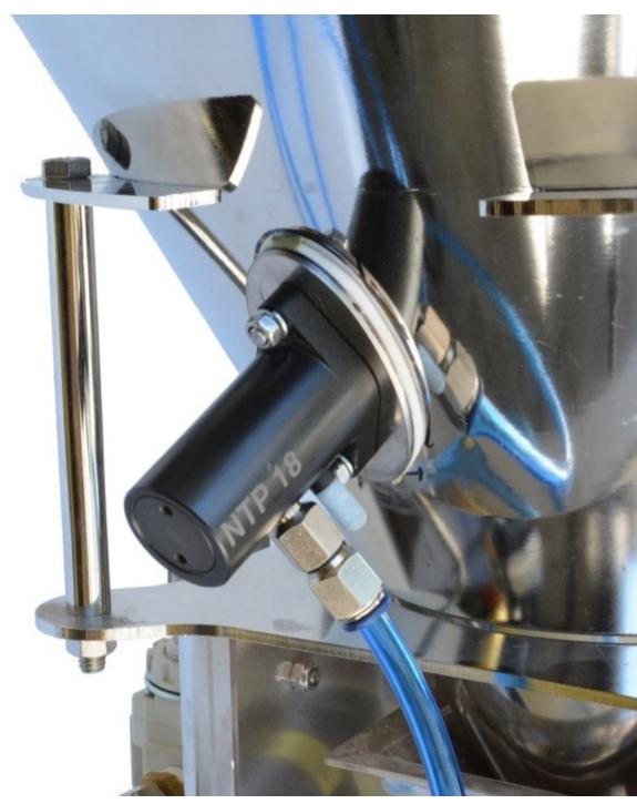
A Martin NTP 18 vibrator mounted on a hopper using the Stick and Shake system.
