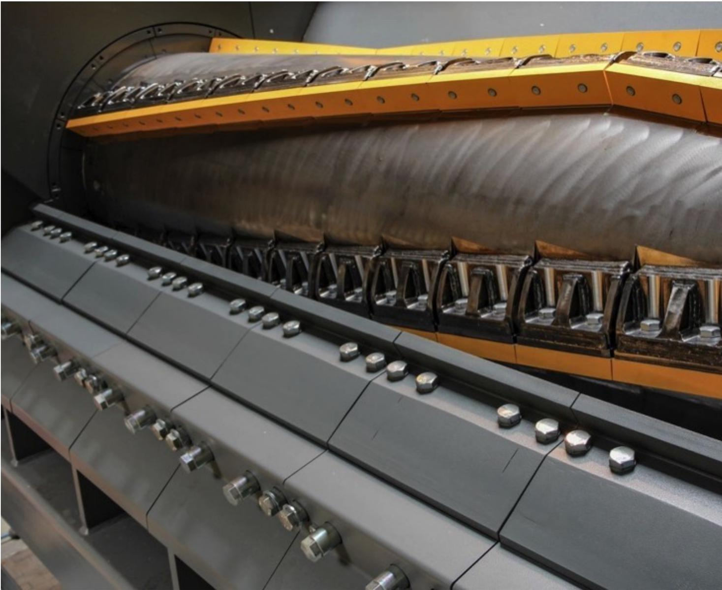
The X-Cutter design is able to deal with large unshreddable items without the excessive downtime that operators typically face with the major repairs needed on high-speed technology.
