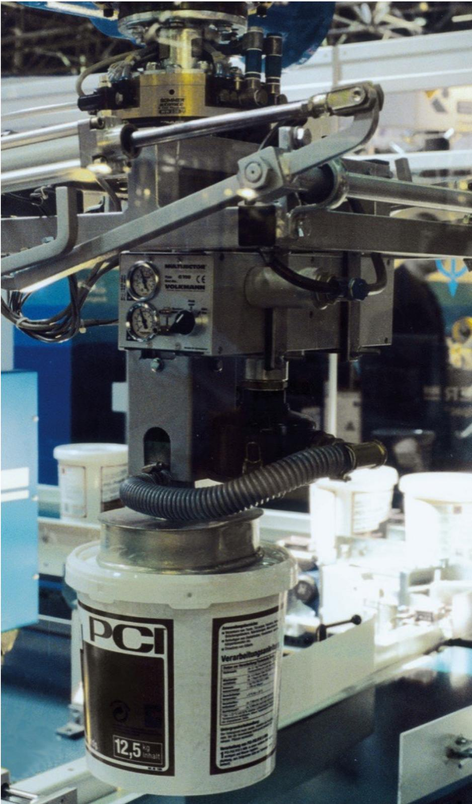
The gripper is specially designed to handle all items with surfaces that need to be suctioned.
