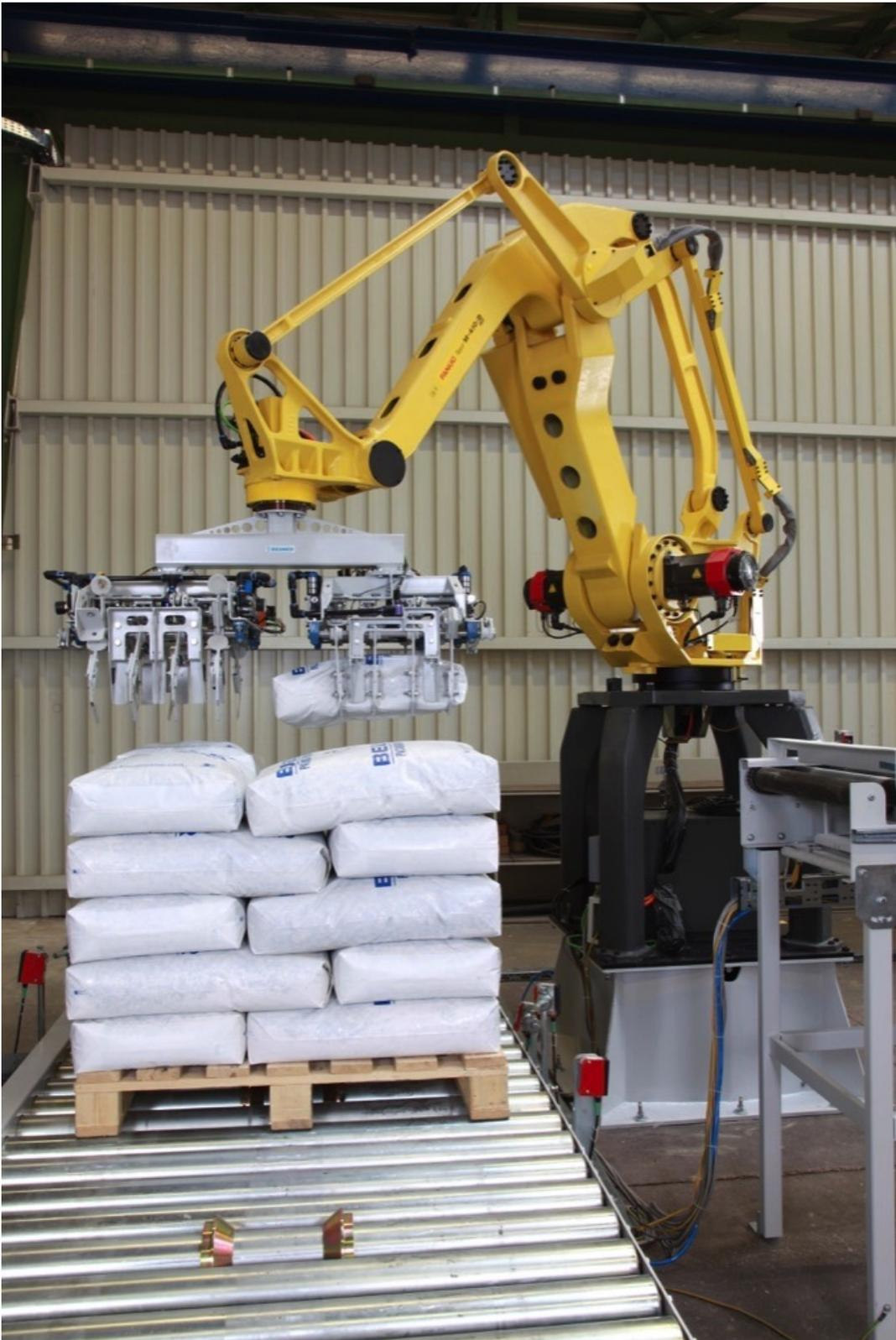
The BEUMER robotpac series palletises and depalletises a wide variety of packaged goods with specially designed gripping systems.
