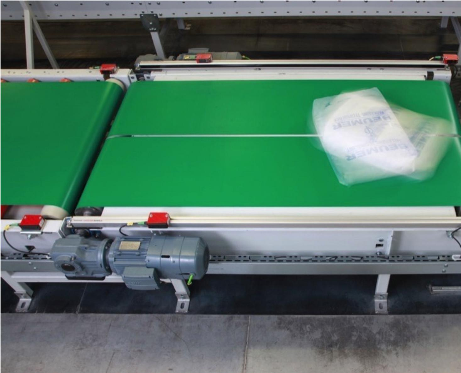
The twin-belt turning device offers a tremendous advantage over conventional turning processes.
