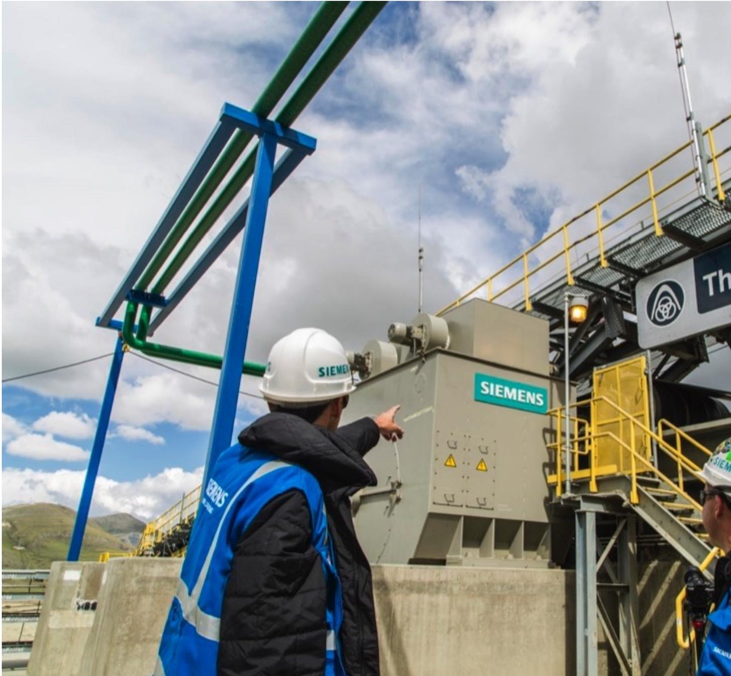
The gearless drive system installed at the Las Bambas Copper Mine includes four low-speed synchronous motors (4.4 MW, 66 rpm) and the associated
