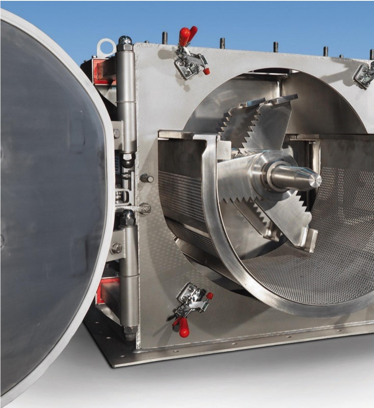
Serrated blades projecting from a rotating shaft whisk material against a contoured grinding screen.
