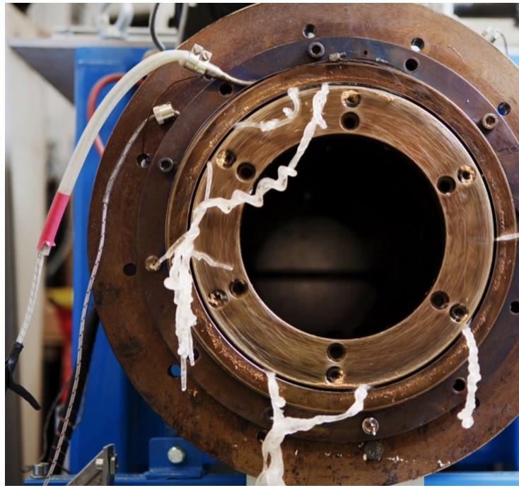
VTT's cylindrical extruder can be used, for example, to turn problematic textiles and plastics as well as food waste into pellets.
