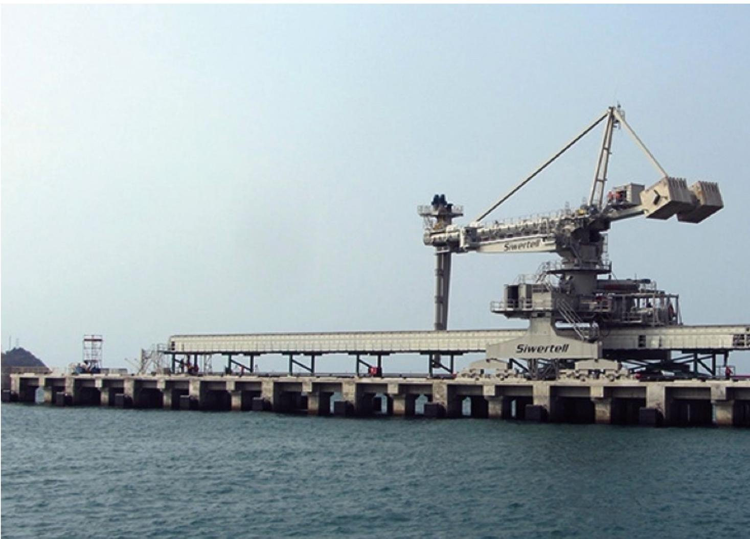
The Siwertell System at Cilegon, Indonesia includes one ST790 D-type shipunloader and two belt conveyors.
