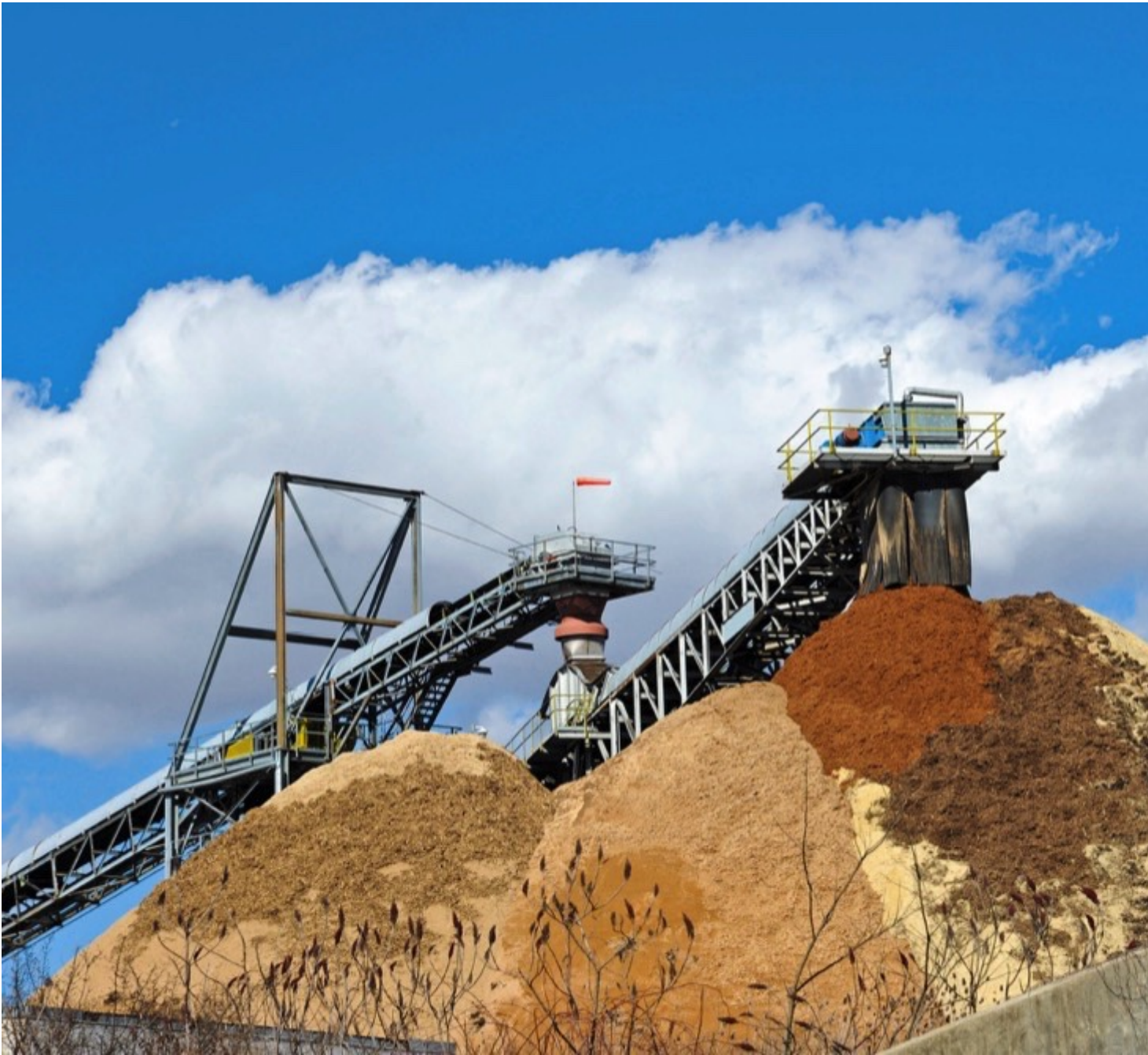
Stacker conveyors dumping wood chips and biomass on a pile. (Mark Winfrey © 123RF.com)
