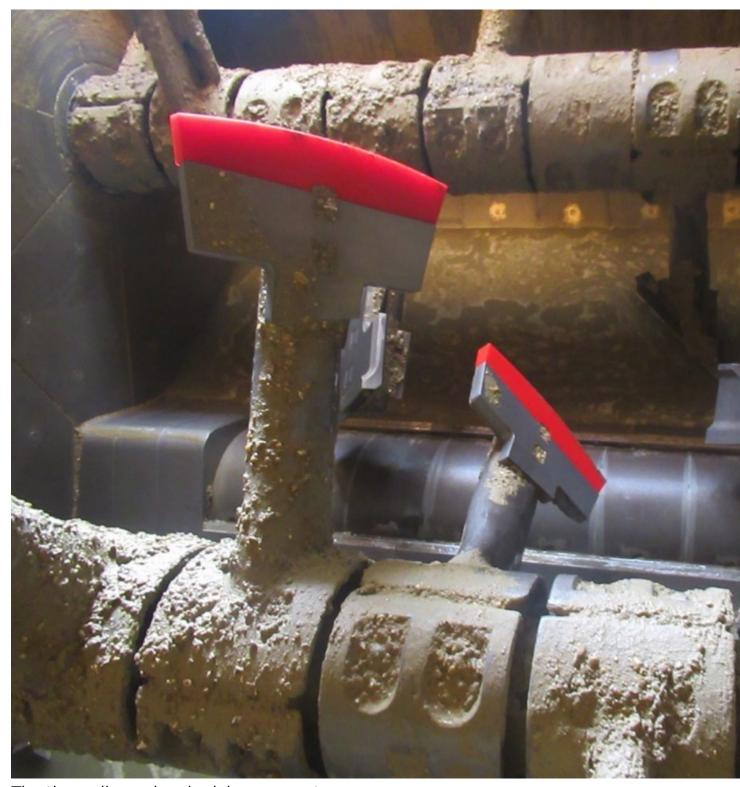
The three-dimensional mixing concept results in an intensive exchange of materials, and shorter mixing cycles with reduced energy consumption.
