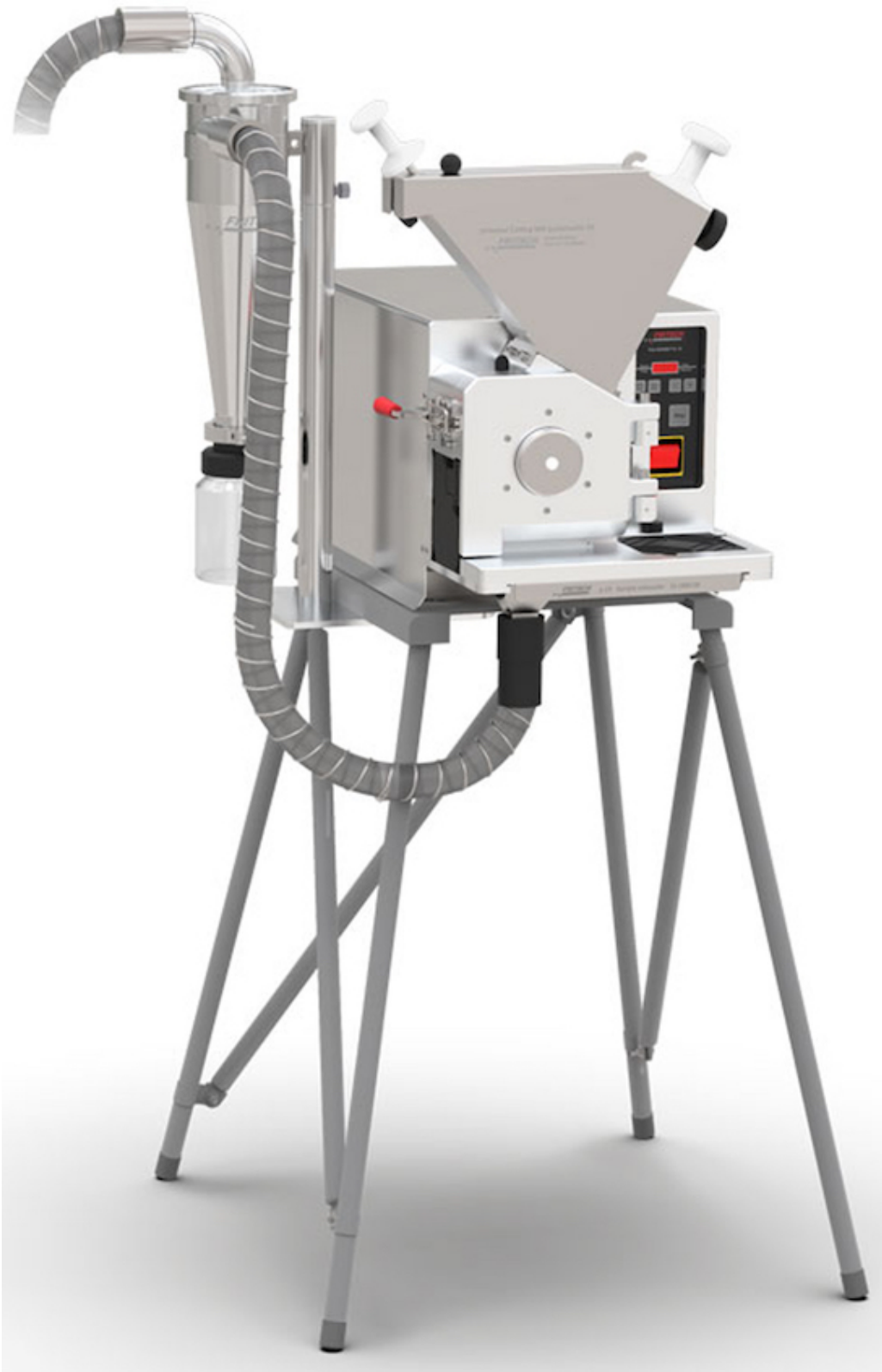
Pulversiette 19 with new Fritsch high-performance cyclone separator.
