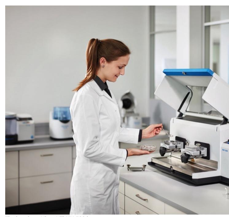
The benchtop Mixer Mill MM 500 by Retsch is suitable for dry, wet and cryogenic grinding of sample volumes up to 2 x 45 ml in one run.
