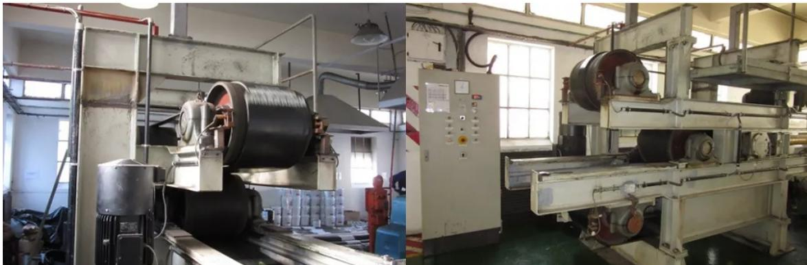
Fig. 6: DIN dynamic splice testing equipment
