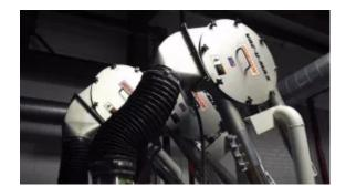
Aero-mechanical conveying systems are space-saving and allow for gentle conveying even for friable products.
