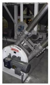
Material is fed to the aero-mechanical system at the conveyors sprocket-end.
