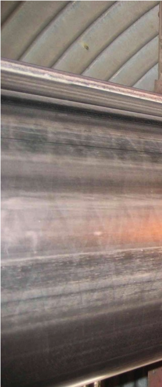
Fig. 12: The new belt contacts all idlers in the carrying strand.
