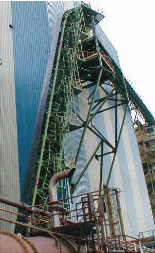
Fig. 10: DSI Snake Sandwich high angle conveyor.
