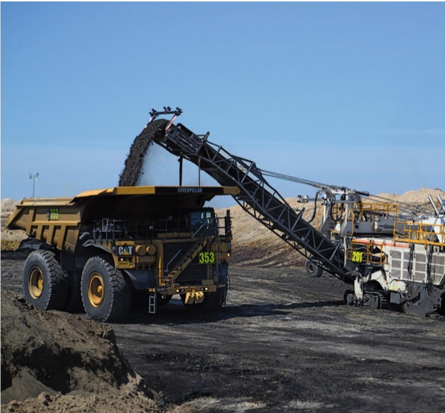
Cutting, crushing and loading in a single pass. Wirtgen surface miner make coal mining simple, economical, eco-friendly and safe.
