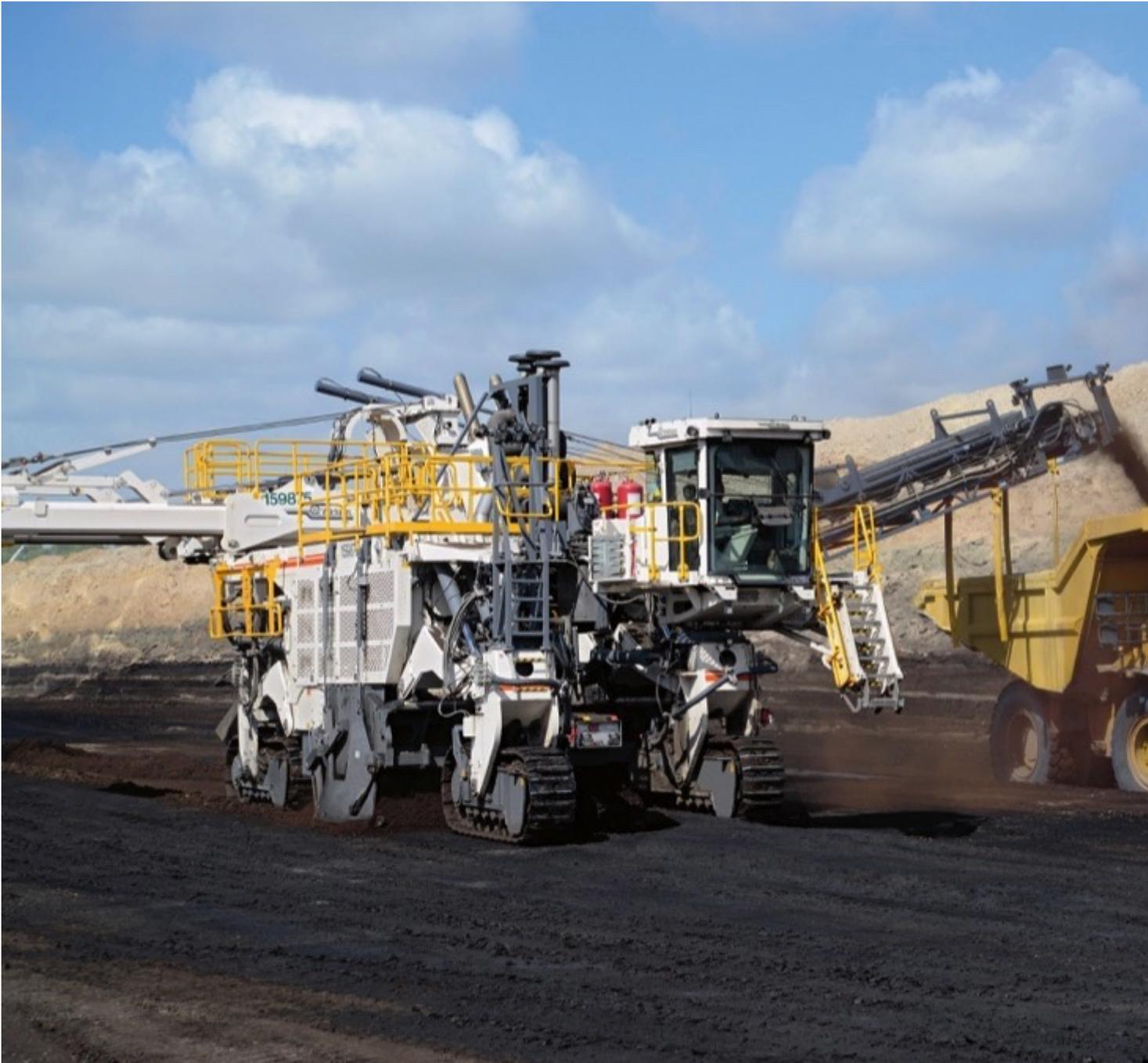
The surface miners loading conveyor can be slewed 90° to either side.
