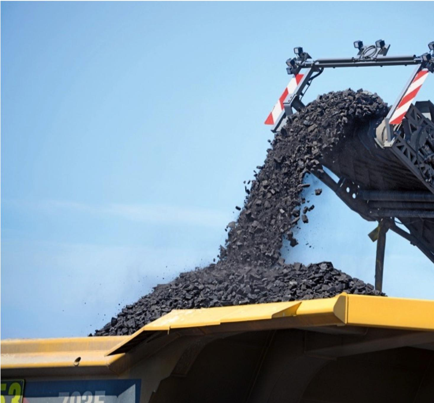
The 4200 SM crushes the lignite to a maximum grain size of 10 cm during the mining process.
