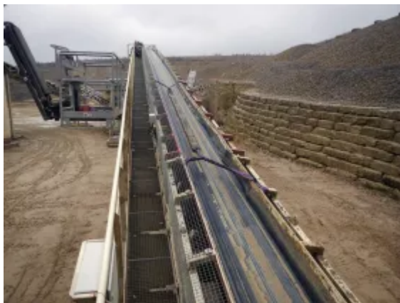
Fig. 1: Adjustment of a belt scale with a test chain.
