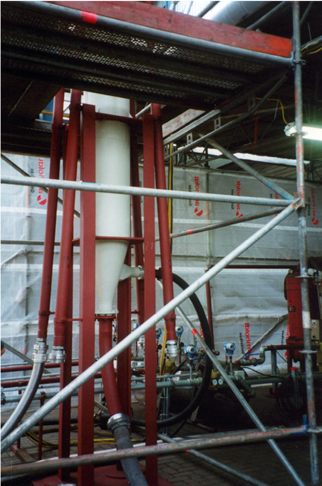
Fig. 13: Pictures of the splitter with connections for single pipes and additional air.
