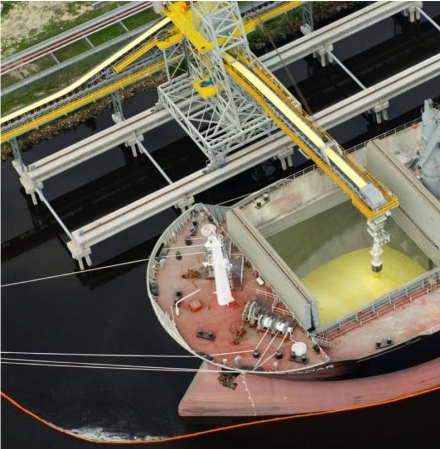
The new Siwertell ship loader will be used for loading prilled sulfur at a rated capacity of up to 1200 tph. (Picture: © Bruks Siwertell)
