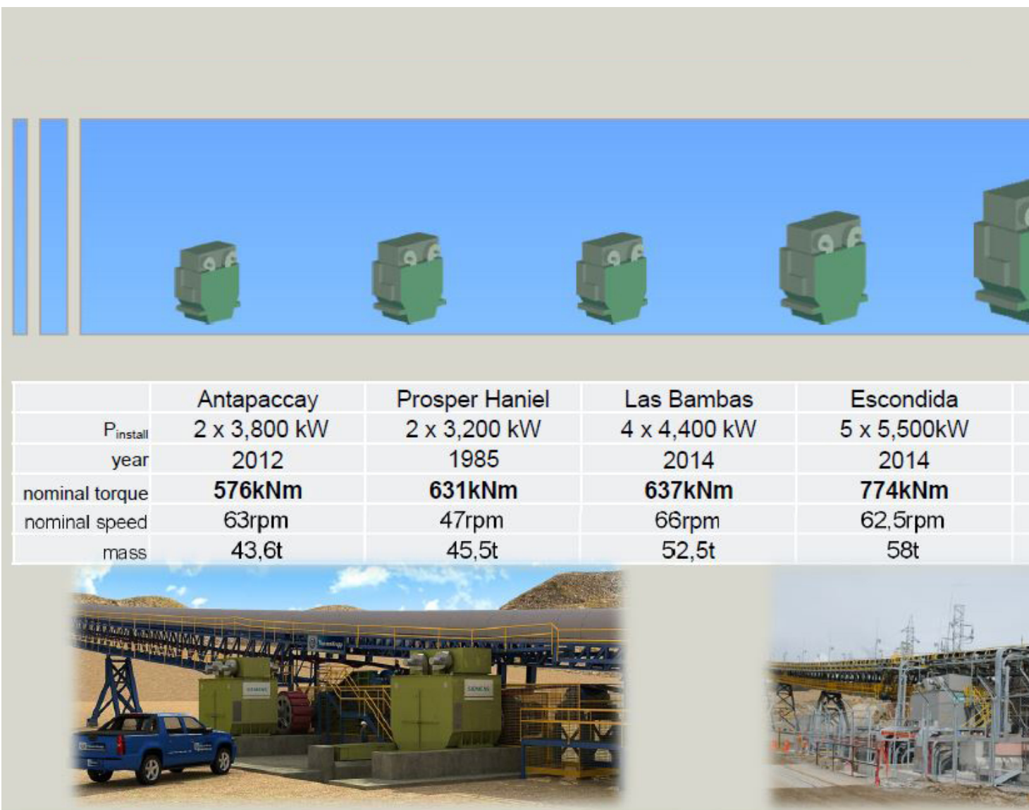
Fig. 6: Development of the Directdrives for belt conveyors. (Picture: © siemens AG)
