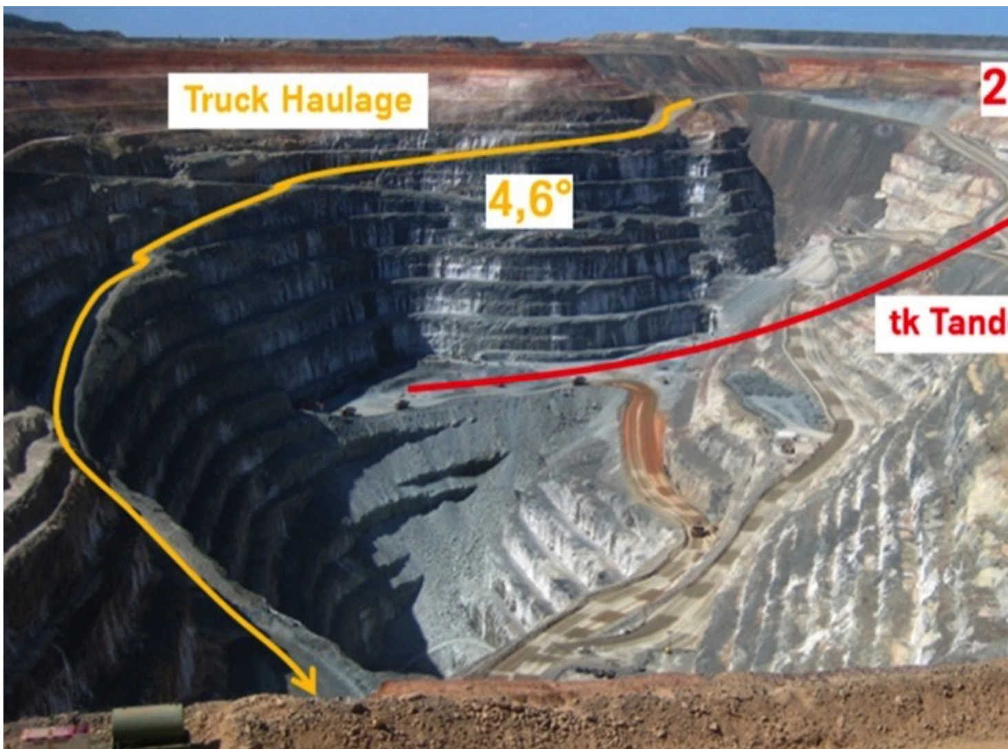
Fig. 1: Alternative ore/mineården haulage in open-pit mines and quarries. (Pictures: © Thyssenkrupp Industrial Solutions - Material Handling)
