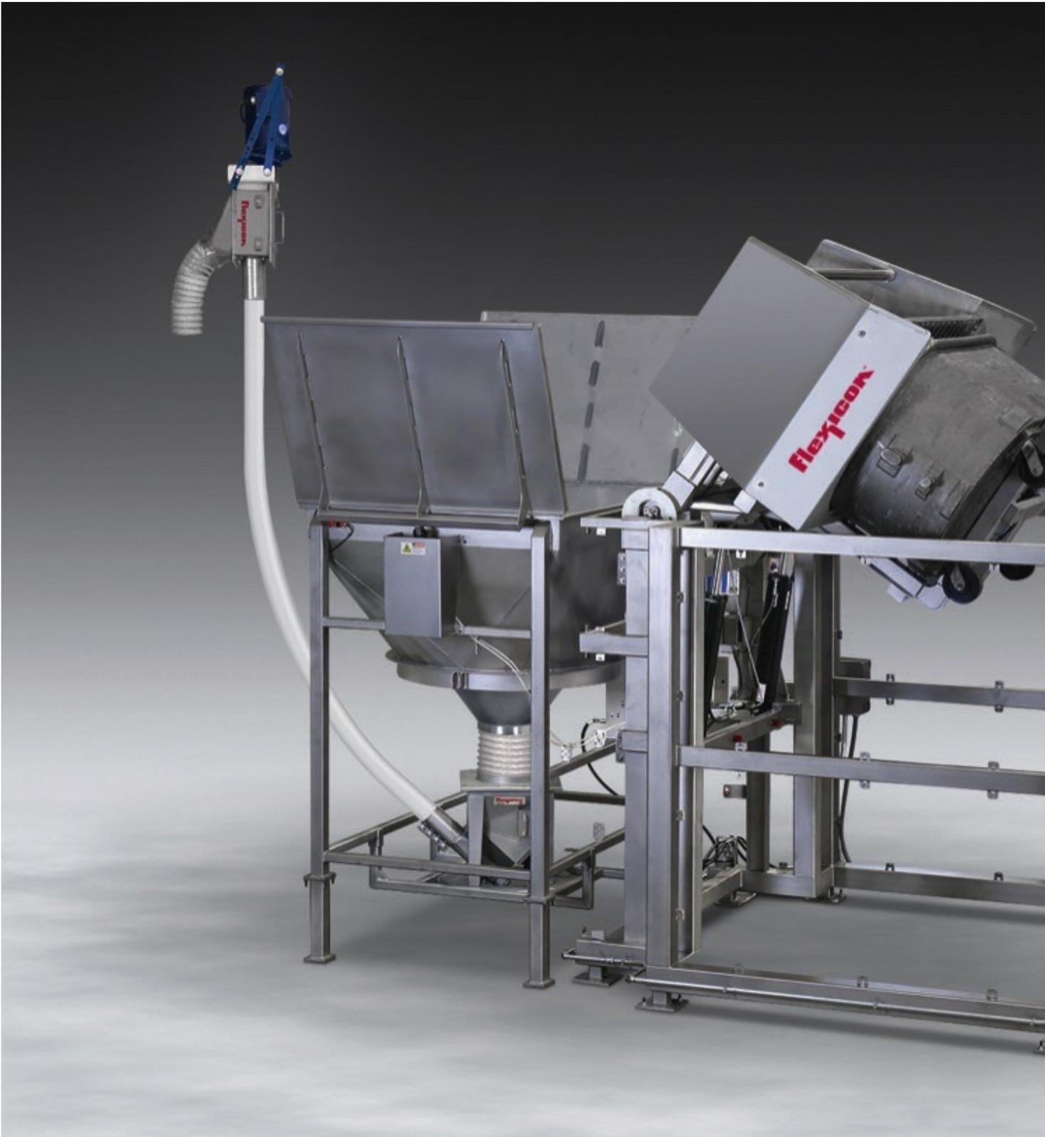
Open-Chute High-Lift Tipper raises and tips wheeled bins weighing up to 1350 kg to a height of 1.5 to 3 metres, charging a 1.7 m<sup>3</sup> hopper and, in turn, a flexible screw conveyor under automated controls.
