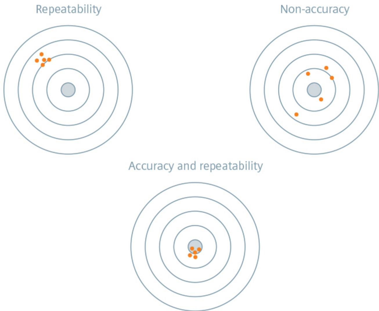
Fig. 3: Repeatability and accuracy are both important issues to ensure reliable readings.
