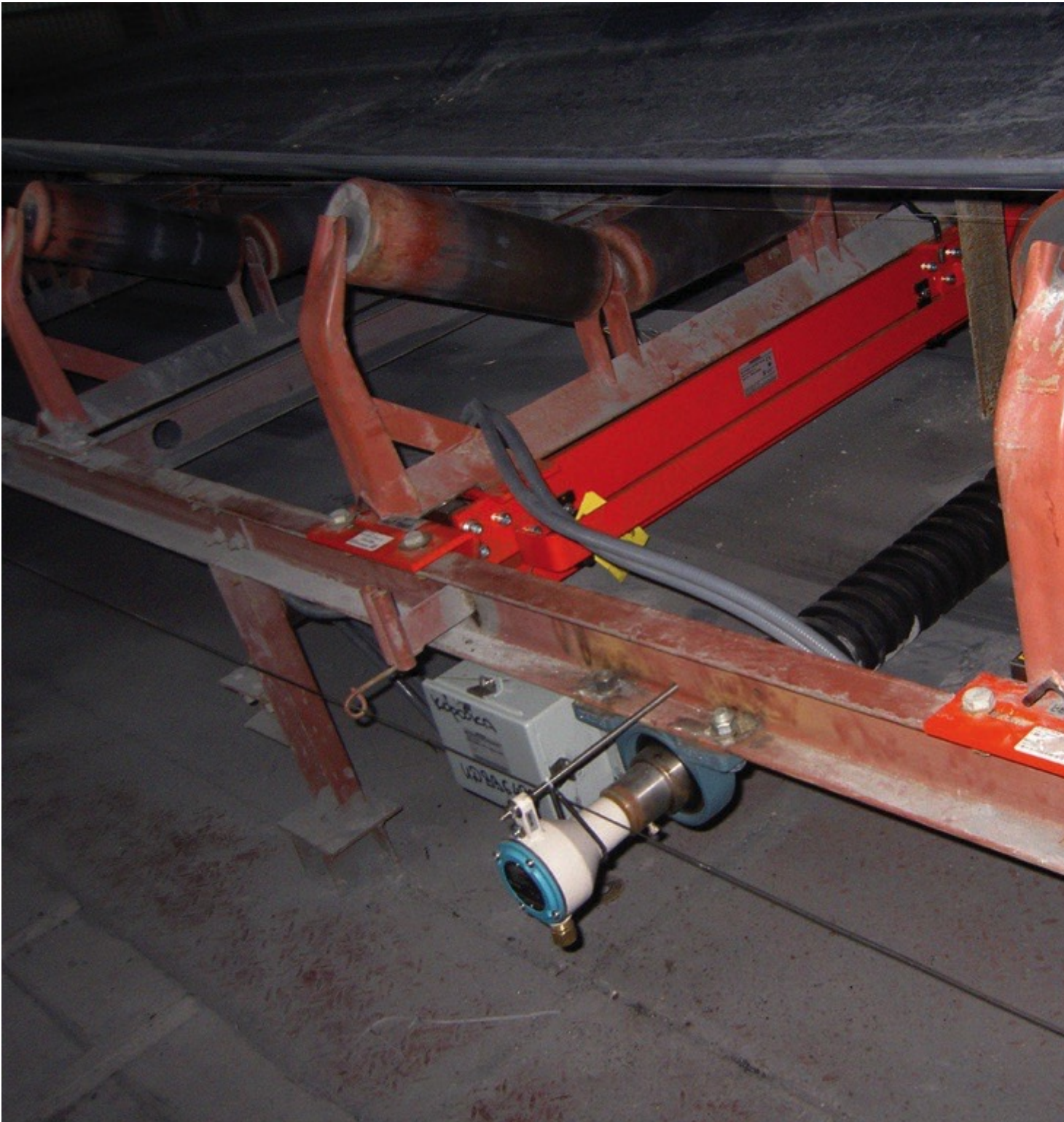
Fig. 1: Installation of a Milltronics MMI belt scale and Sitrans WS300 speed sensor. (Pictures: © Siemens AG)
