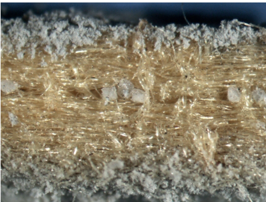
Fig. 4: Contamination from the clean gas side.
