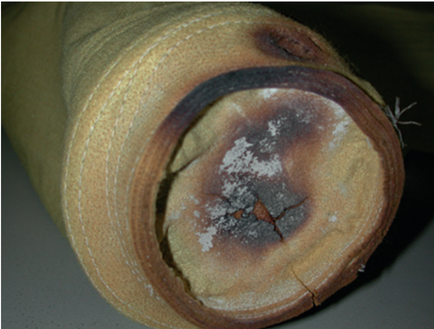
Fig. 5: Shrunken bag bottom as a result of high hopper dust levels.
