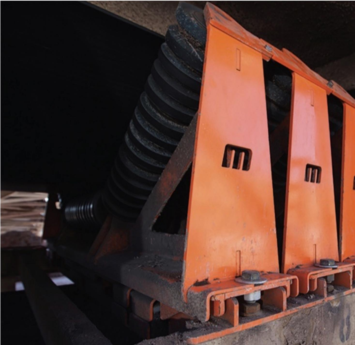
Track-mounted idlers allow easy access for quickly swapping out seized rollers.
