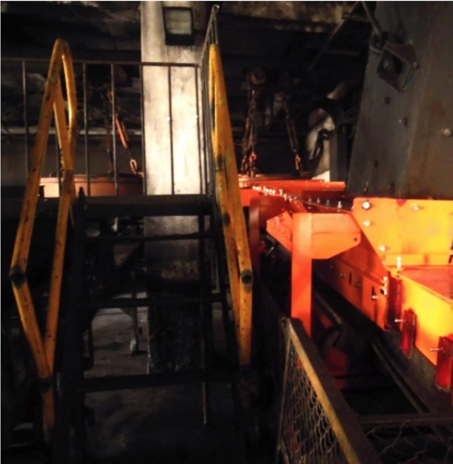
A hatch over the tail pulley allows staff to easily detect entrapped material.
