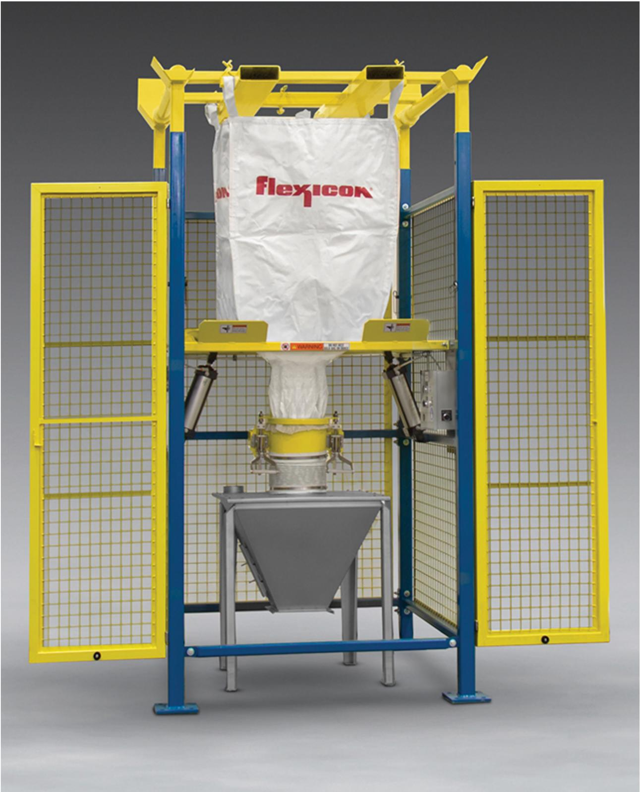
Steel safety enclosure of BULK-OUT®
