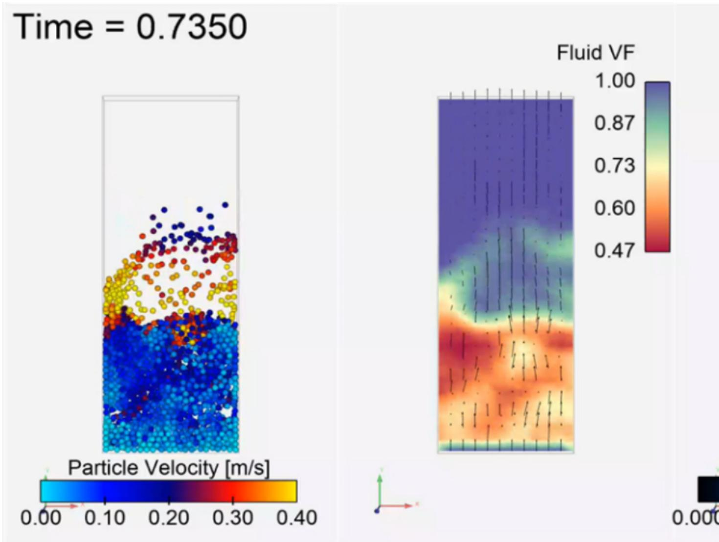
Fluidized bed heating and drying wet particles using EDEM-Fluent coupling (Courtesy of Astec).
