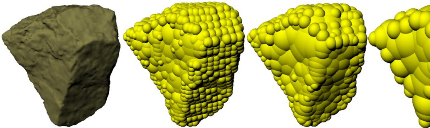
Creating complex shapes in EDEM is now an automated process with the Sphere Fitting Tool.
