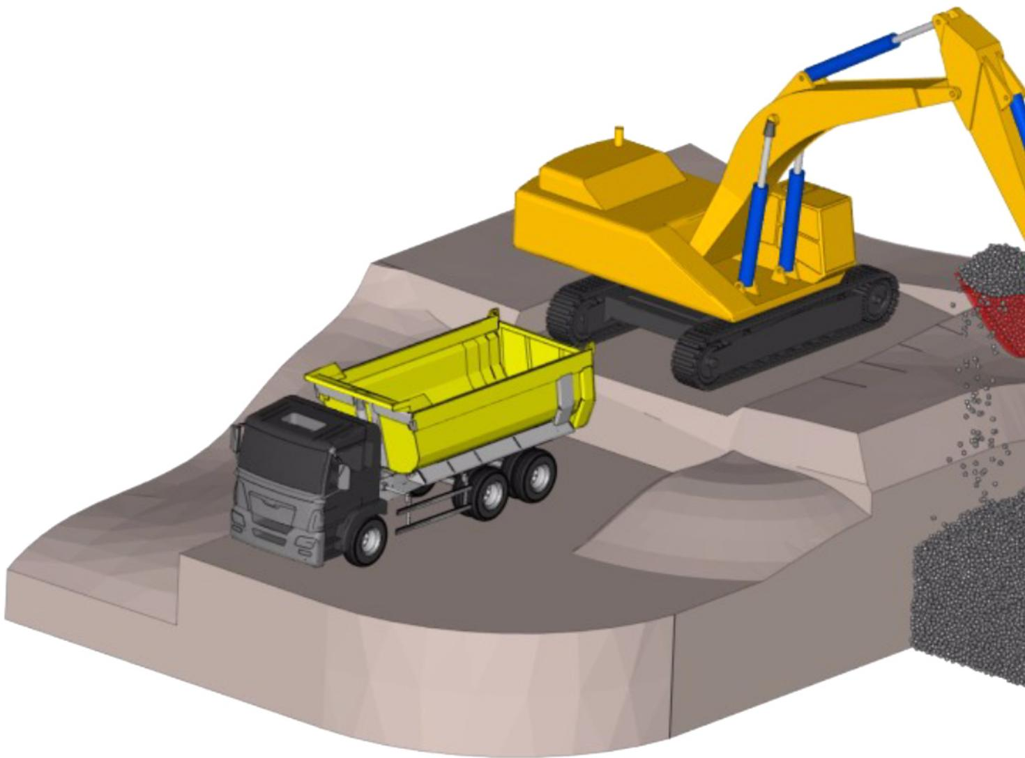
EDEM-MotionSolve co-simulation provides the capability to model and visualize dynamics of equipment movement and examine how loads exerted by bulk materials are distributed throughout a mechanical system.
