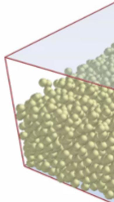
A material block of particles can be automatically inserted into a simulation at regular time intervals to replicate the outflow from a physical system.
