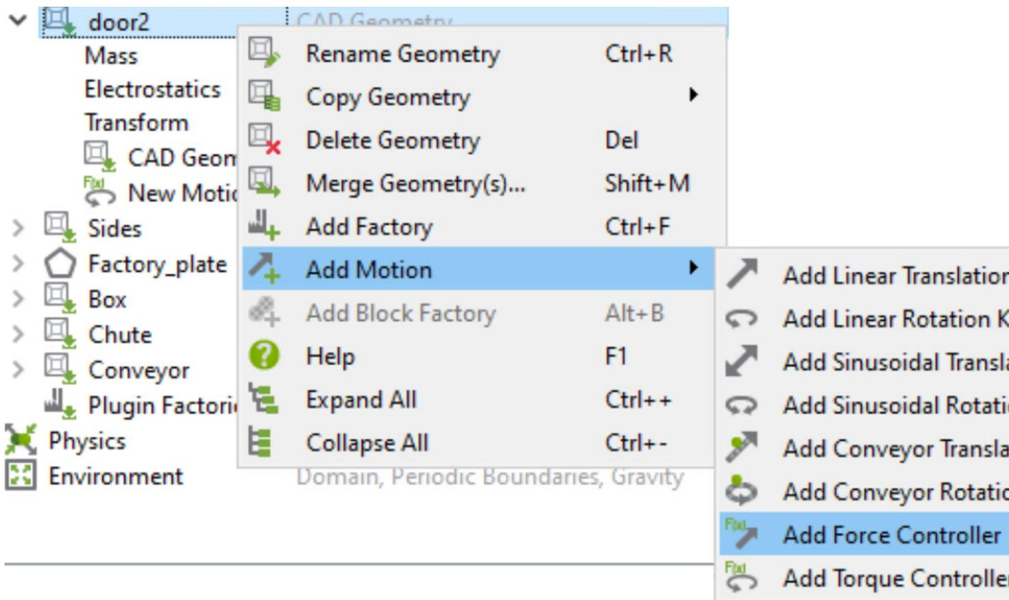
Motions to geometries that occur due to forces or torques being applied can be easily introduced.
