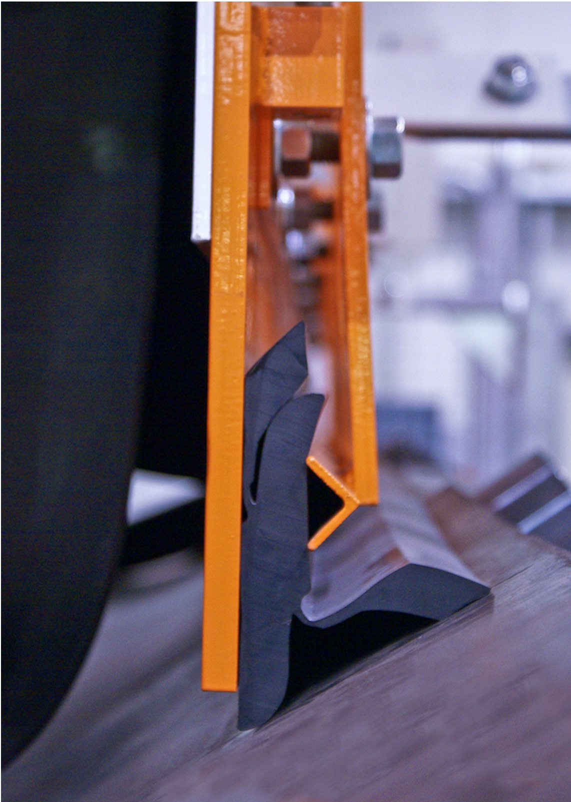
Fig. 5: The primary seal is clamped to the steel skirtboard and a secondary “outrigger” strip captures the fines. (Picture: © Martin Engineering)
