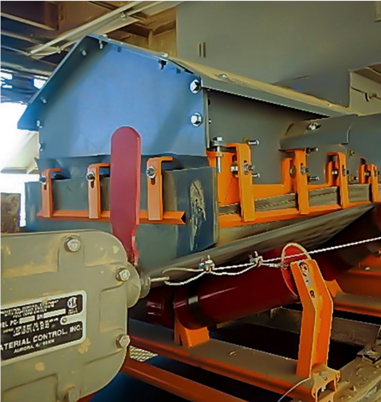
Fig. 4: The modular chute wall allows easy installation of skirt boards and stilling zone components to manage dust. (Picture: © Martin Engineering)
