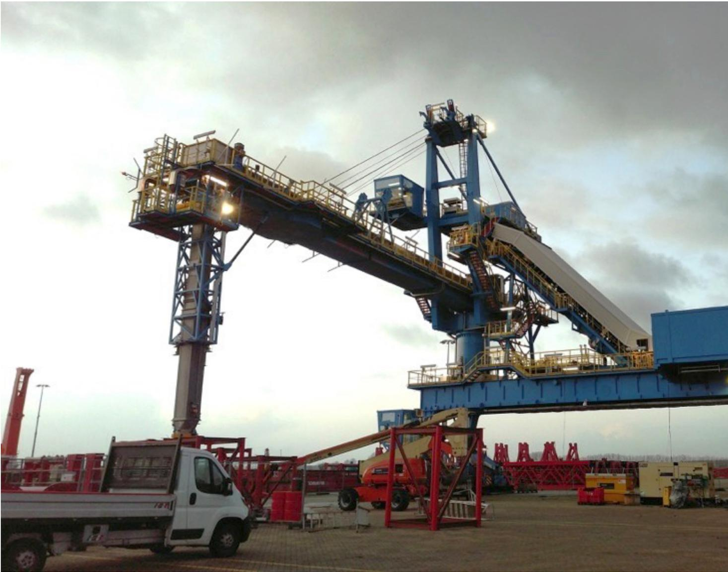
The DSI Sandwich high angle conveyor will transfer urea and amidas prills at a rate of 600 t/h at a 45° angle.
