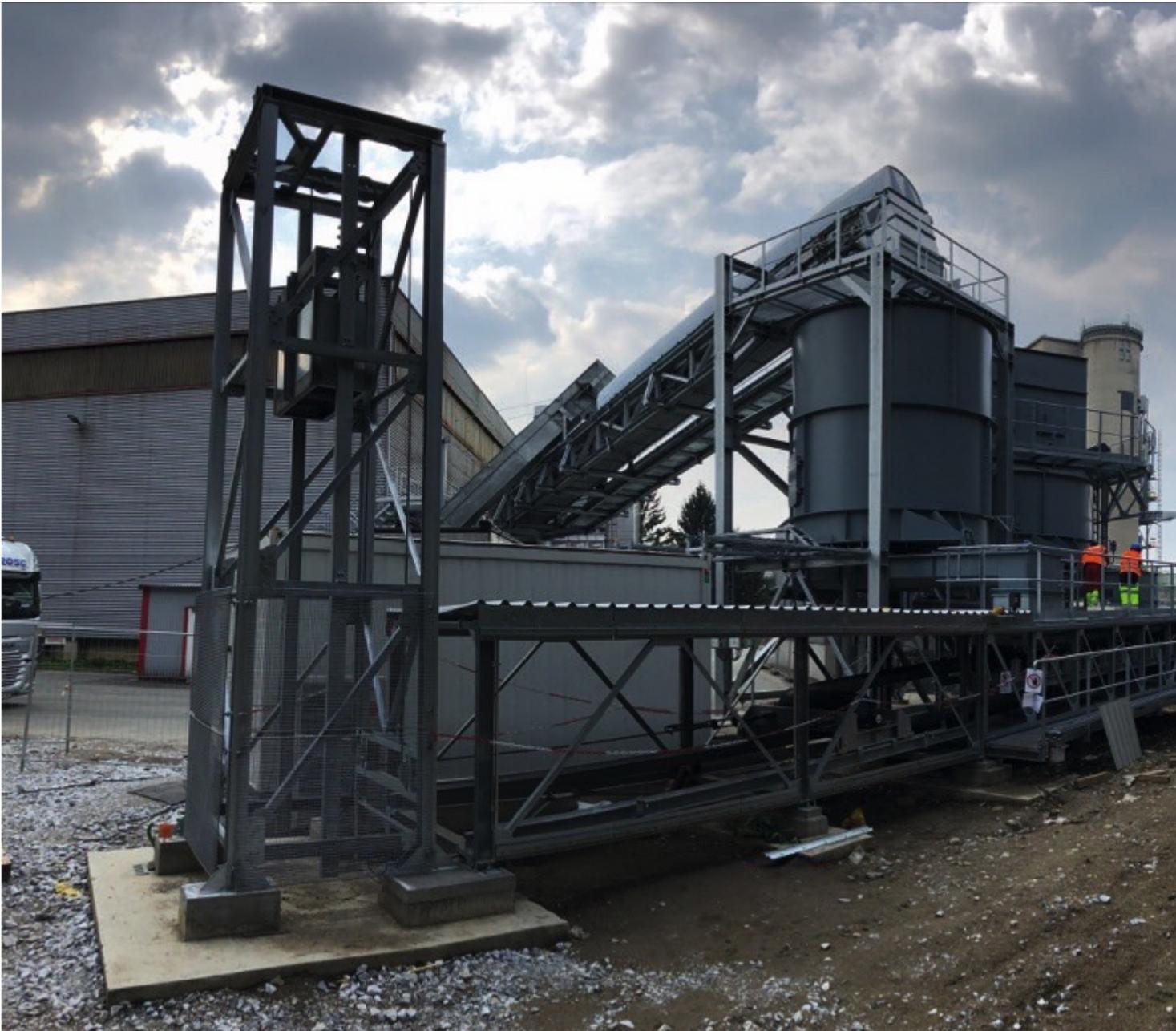
The high-precision system is used in the energy-intensive production of cement. (Picture: @BEUMER Group GmbH & Co. KG)
