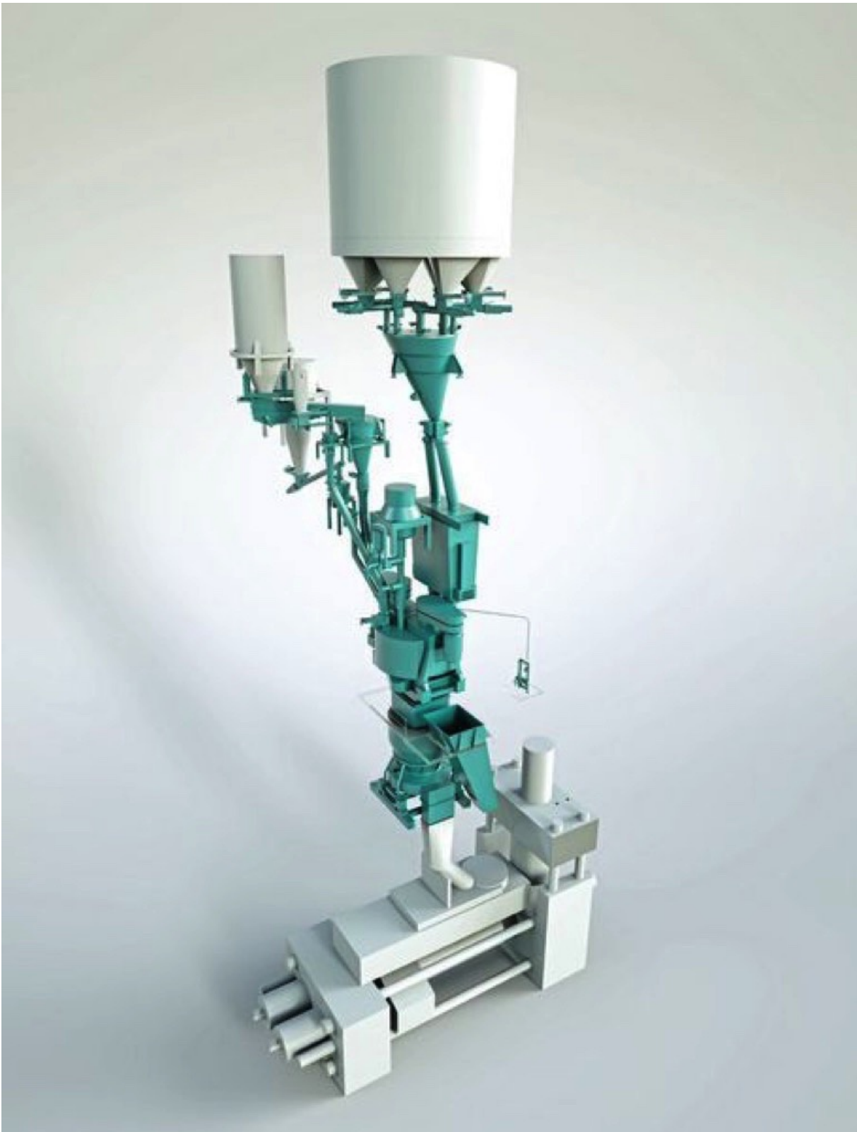
Eirich plant layout for the preparation of graphite electrode compounds.
