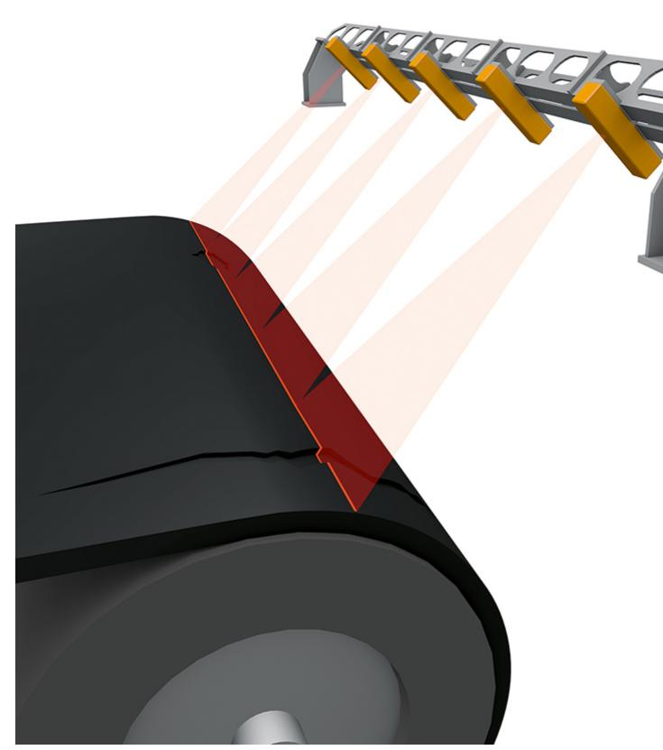
The mobile inspection system Conti SurfaceInspect scans the entire conveyor belt surface by means of ultra-modern line laser technology. (Pictures: ©ContiTech)
