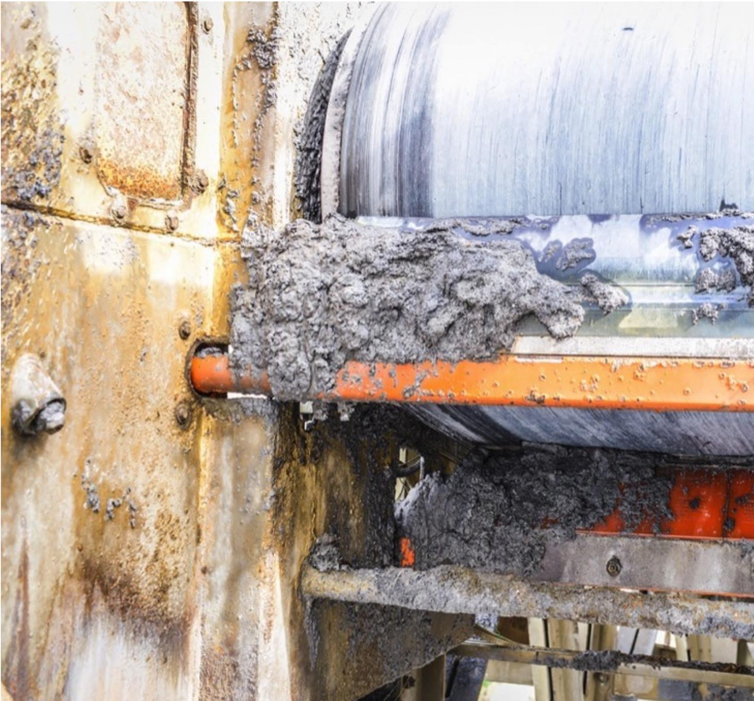
The carryback had the consistency of toothpaste, adhering chunks of aggregate to the belt and causing damage to pulleys and headers.
