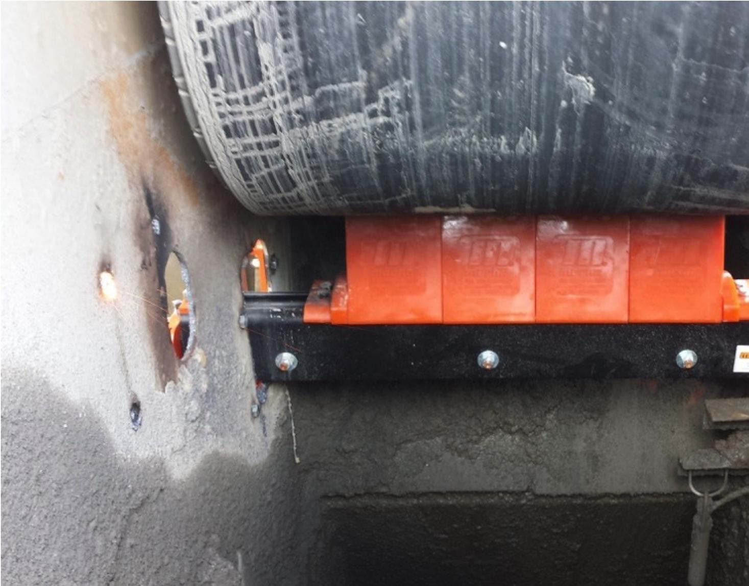
Sixteen additional secondary belt cleaners were attached behind the header, equipped with tungsten tipped blades.
