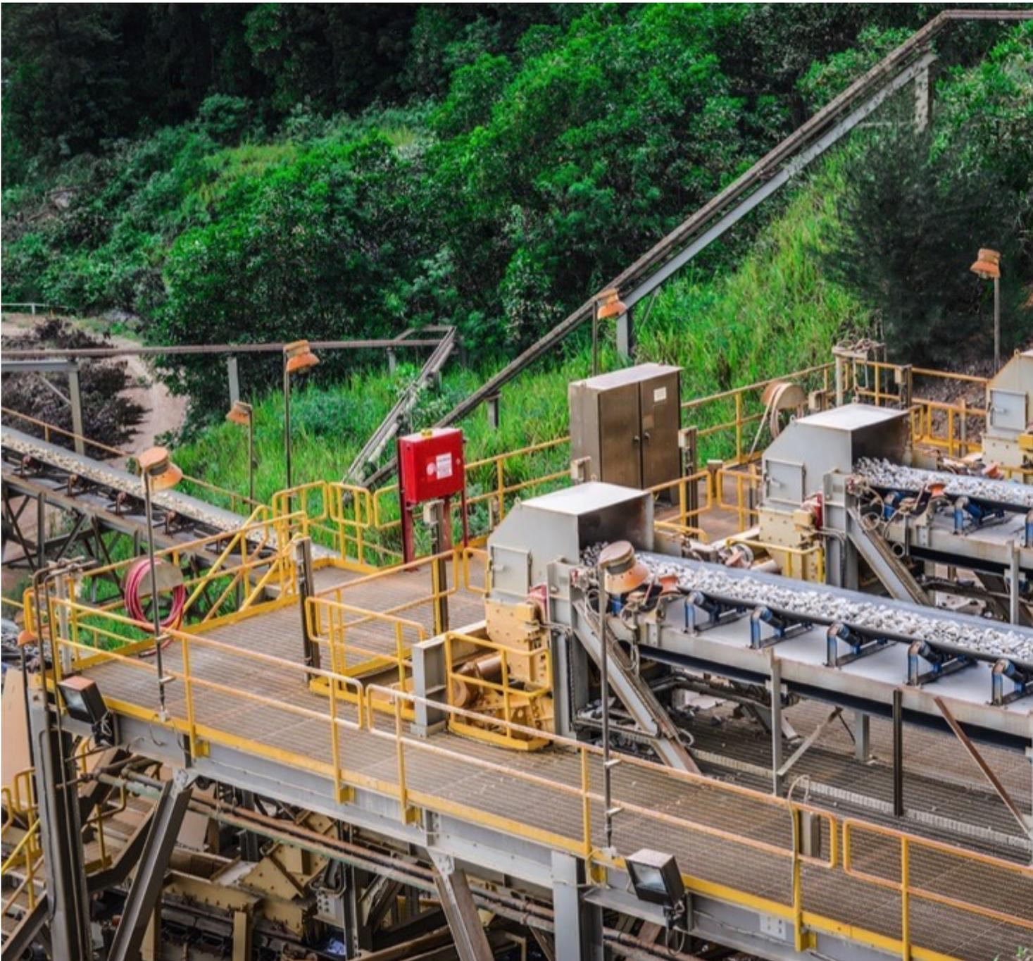
The original conveyor belt cleaners could not manage the overburden, resulting in carryback that caused
