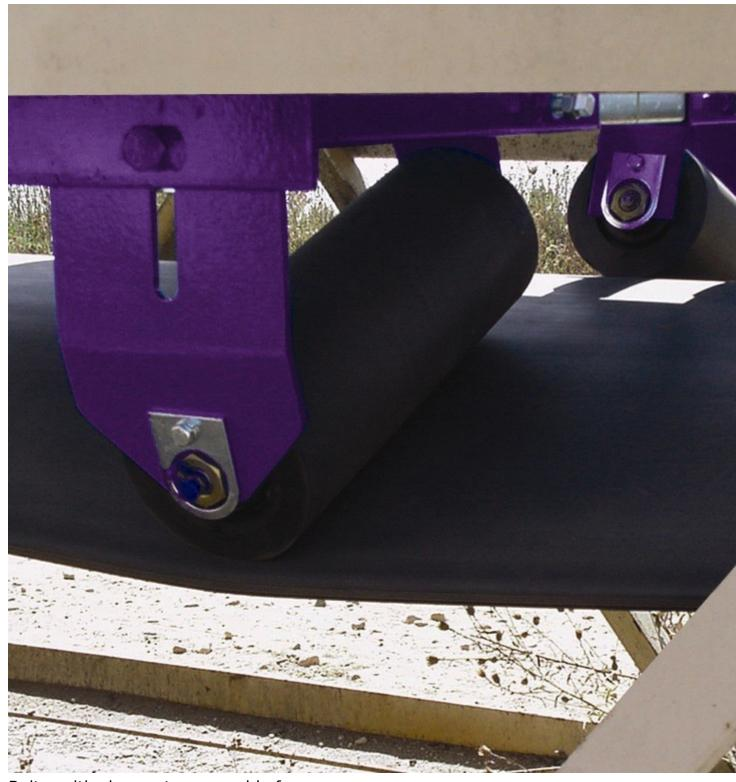
Belt positioning systems provide for a straight run of the conveyor belt, thereby ensuring a proper material flow. (Pictures: © Flexco)
