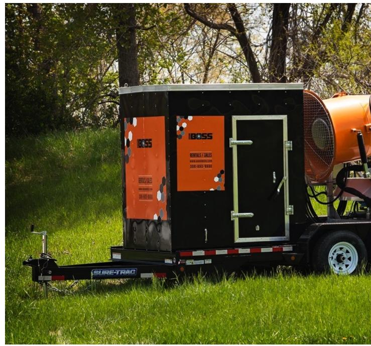
Each liquid-bearing component is insulated, heat traced or both, ensuring effective operation during cold weather.
