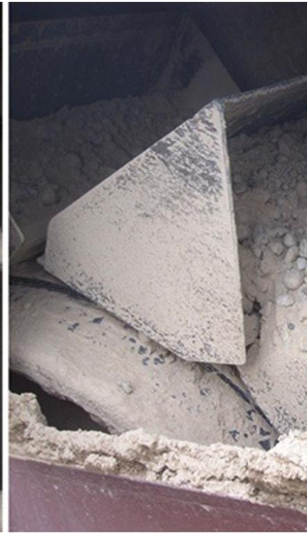
Belt bucket elevator type BWG-GK for coarse grain: the narrow, overlapping bucket configuration permits the belt to disappear entirely behind the buckets. No coarse material will be thrown behind the backs of the buckets, even after stoppage.
