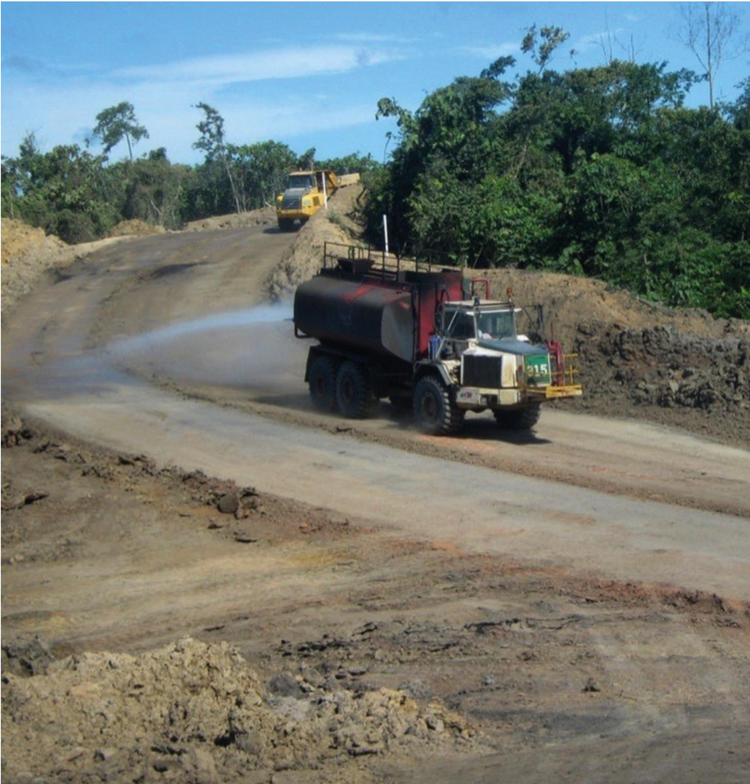
To reduce the amount of dust raised by the overburden-transport haulers the roads need to be watered. This is done by converted articulated haulers.
