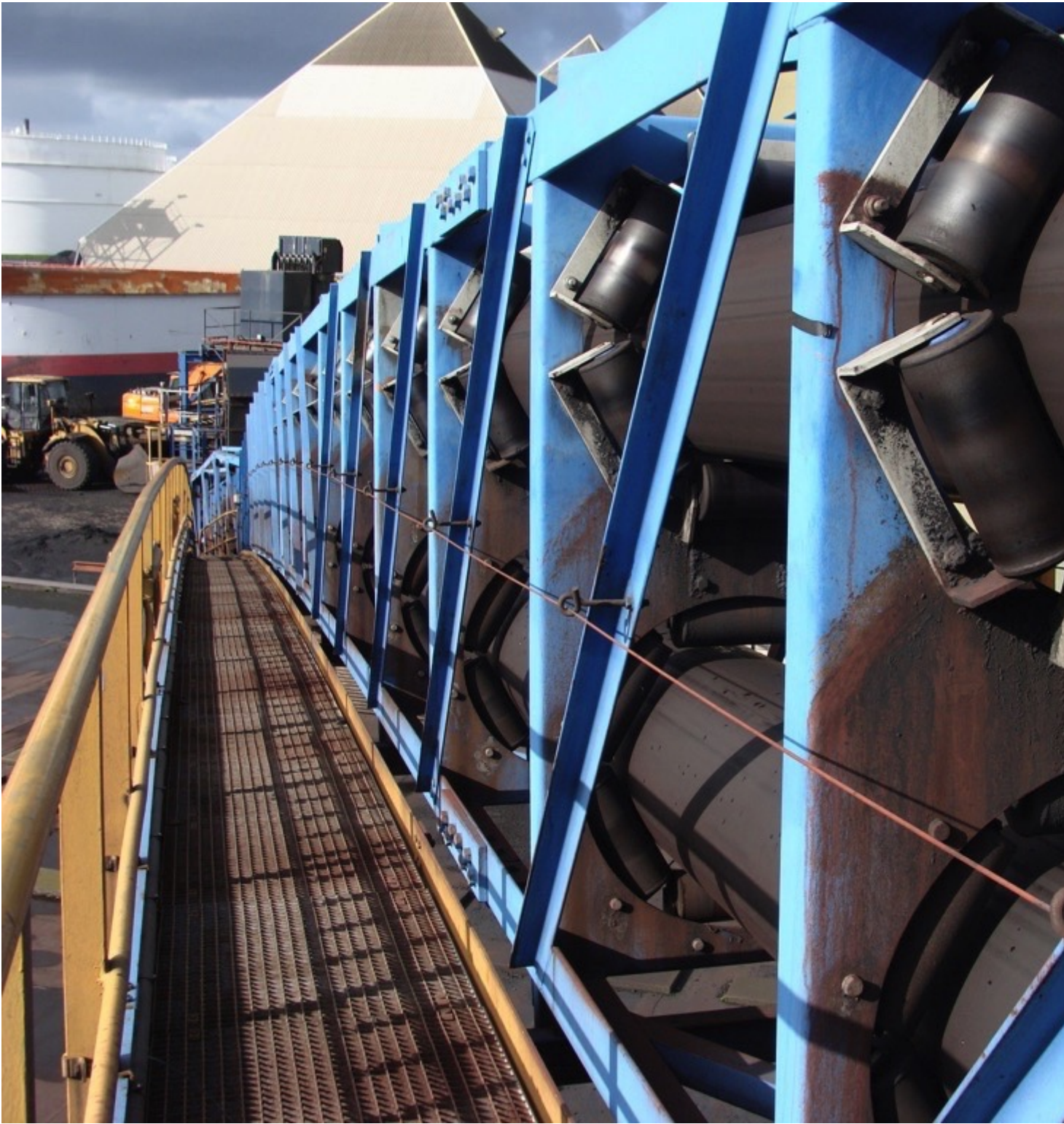
Fig. 1: Pipe belt conveyor in Laurens haven Terminal, European Bulk Services (EBS) B.V., the Netherlands. (Picture: © M.E. Zamiralova, Delft Univ. Technol.)
