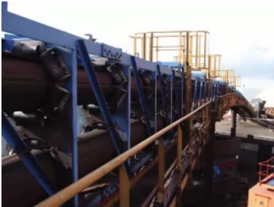
Fig. 1: Pipe belt conveyor in Laurenshaven Terminal, European Bulk Services (EBS) B.V., the Netherlands. (Picture: © M.E. Zamiralova, Delft Univ. Technol.)
